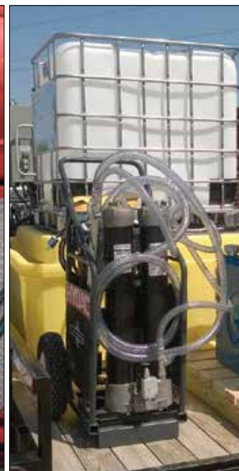
OFS Filtration Station with HPU.
