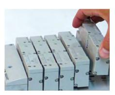
Plug-and-play valves can be replaced quickly and easily, helping to prevent long interruptions to production. ▶ p14
