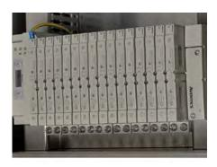
CHARMs node and Electronic Marshalling provide simple connection and integration to the control system enabling faster start-ups. ▶ p13
