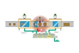
Zoned Safety capability enables isolation of up to three safety zones on a machine from one single valve system, improving productivity, and reducing cost and complexity.
