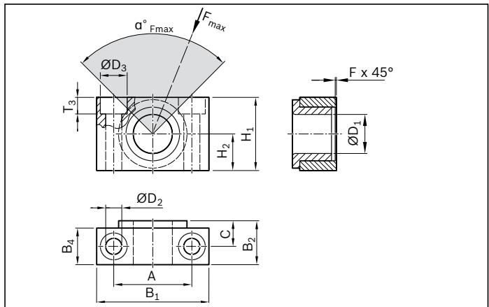
**Note:** Bearing for trunnion for vertical load; if  $\alpha F_{max}$  is not complied with, a positive lock must be added
