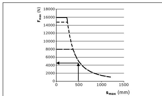
$F_{\max}$  in table "Drive data" with motor attachment via timing belt side drive:  $F_{\max} = 11,400$  N
