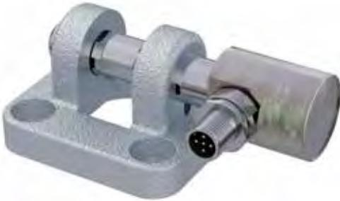
If your application requires precise load sensing, there is a clevis bearing block version with force measuring bolt available for this purpose. This option can be selected both at the piston rod end connected to the spherical rod end bearing, and at the timing belt side drive.
