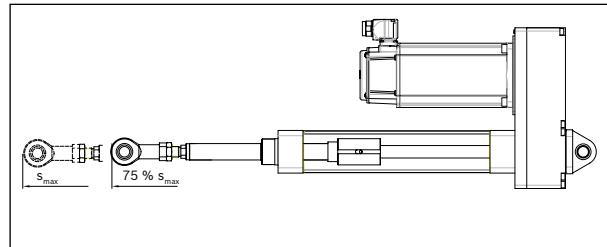
Note: In this installation case, the cylinder is loaded by its own weight when mounted in a horizontal position. Thus, the piston rod may be extended horizontally only up to 75% of  $s_{\max}$ .
