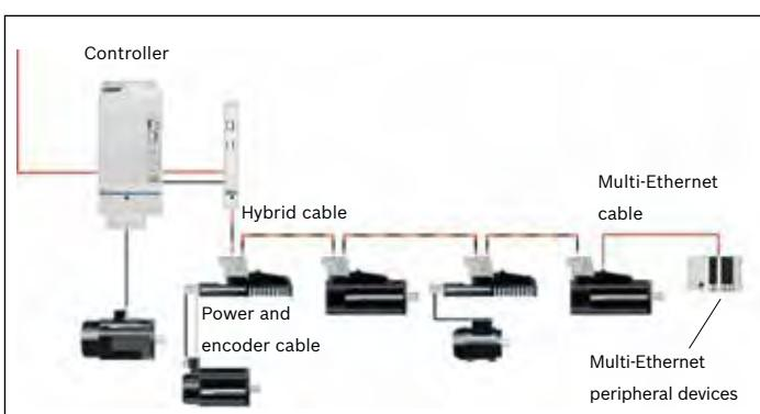
Up to 20 IndraDrive Mi in a string – these motor-integrated servo drives (KSM) and servo drives close to the motor (KMS) are freely combinable. Additional IndraDrive Mi-strands can be integrated via further KCU.
