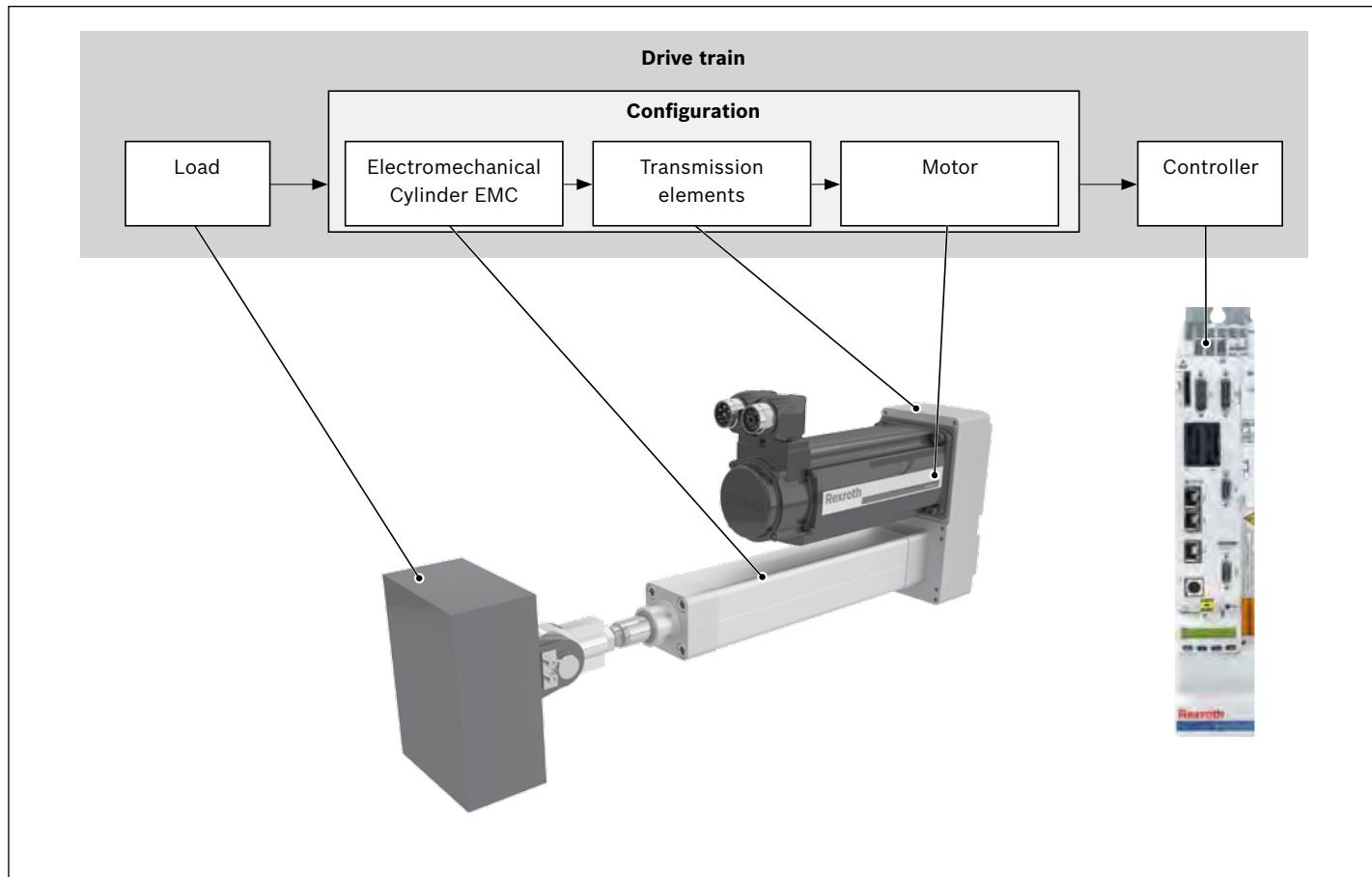
The correct dimensioning and assessment of an application requires structured consideration of the drive train as a whole. The basic element of the drive train is the configuration – comprising the Electromechanical Cylinder EMC, the transmission element (coupling or timing belt side drive) and the motor, which can be ordered in this constellation as per the catalog.
