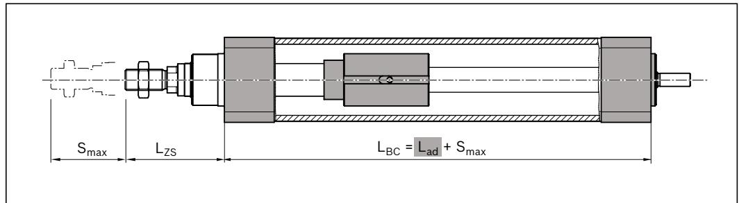
The cylinder can be adapted to the available installation space by mounting the motor as an extension to the axis (mount and coupling) or parallel to the axis (timing belt side drive). The type of motor attachment chosen also has an effect on the technical performance data and the selectable mounting methods.
