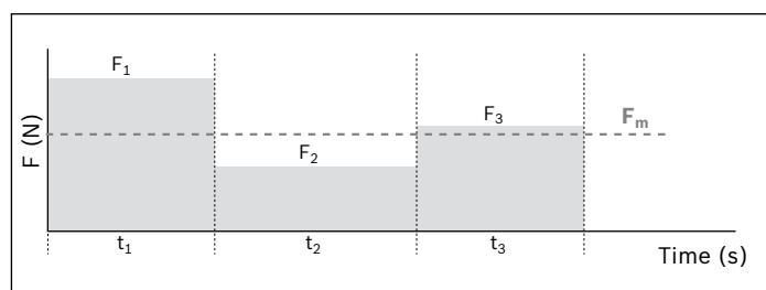
$$F_m = \sqrt[3]{|F_1|^3 \cdot \frac{|v_1|}{v_m} \cdot \frac{t_1}{t_{\text{total}}} + |F_2|^3 \cdot \frac{|v_2|}{v_m} \cdot \frac{t_2}{t_{\text{total}}} + \dots + |F_n|^3 \cdot \frac{|v_n|}{v_m} \cdot \frac{t_n}{t_{\text{total}}}}$$
