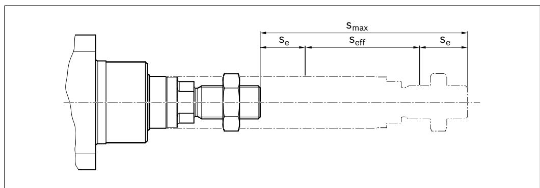
For structural design reasons, the overall length of the cylinder is greater than the maximum travel range ( $s_{\max}$ ), as it includes the length of components such as the screw drive nut and the bearings (represented by  $L_{ad}$ ), in addition to the travel range. The measurement  $L_{zs}$  describes the position of the piston rod in the retracted position.
