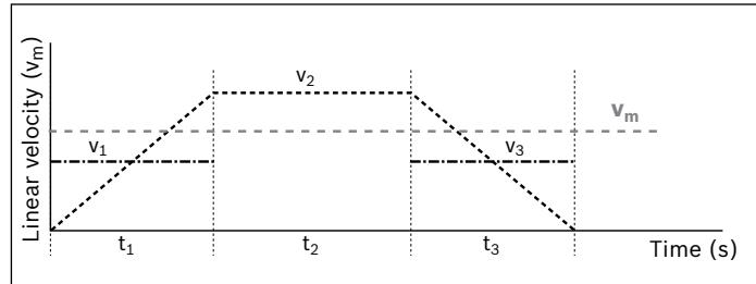
**When the linear speed varies, the average speed  $v_m$  is calculated as follows:**
