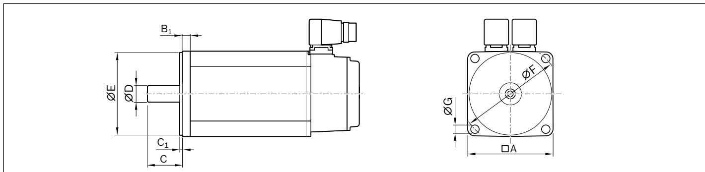
The dimensions queried result in a unique “motor geometry code”:
