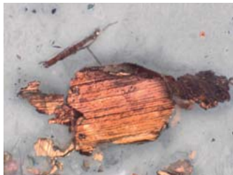
◀ Copper particles, 500 x
