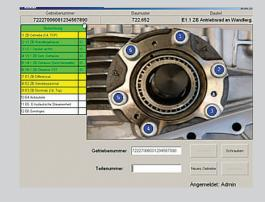
Easy-to-embed images in the worker guidance display show the correct bolt tightening sequence for multi-bolt operations. It indicates bolts that have been tightened and bolts that still need to be tightened. The worker guidance display provides real-time feedback on torque, time, and angle, enabling visual control of the production environment.
