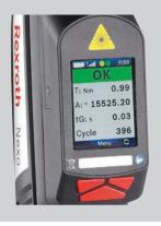
The permanently embedded browser-based software for wireless NEXO tools is icon based and doesn't require a computer to program it. This software can be accessed with any browser on any smart device that is connected to the internet. It allows 1024 programs to be created with 20 steps per program, and monitoring limits are possible for each step in the rundown. Additionally, the NEXO can store up to 10,000 rundown results, which can be viewed on the tool.
