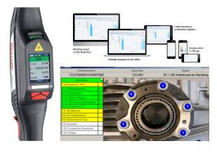
Rexroth offers numerous software options for its spindle tools, handheld tools, and wireless tools. They also offer and maintain a software development platform, IndraLogic, for PLC programming. With this software, programmers can control all of the discrete inputs and outputs in station control and tightening systems.
